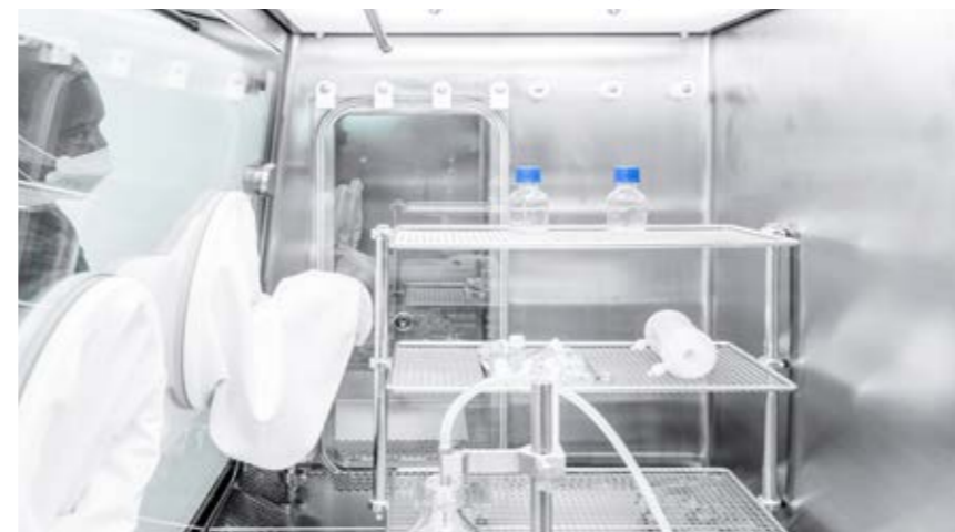
Interior view: Material transfer lock (MTC) with pneumatically sealing sliding door
