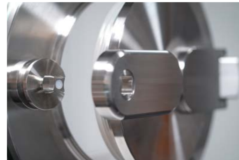
Handling and transfer solution for autoclaved rotary piston pumps in the isolator. With so-called peak devices, the rotary piston pumps can be installed without material product contact.
