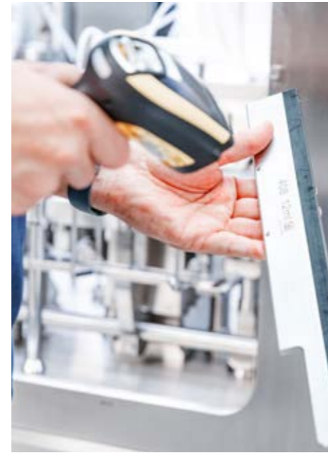
↑ Before installation, format parts are scanned. Systems are therefore completely equipped with the correct format parts and the correct installation order is followed.
