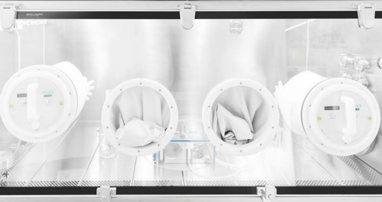
↑ STISO work chamber in standard version with four glove ports
