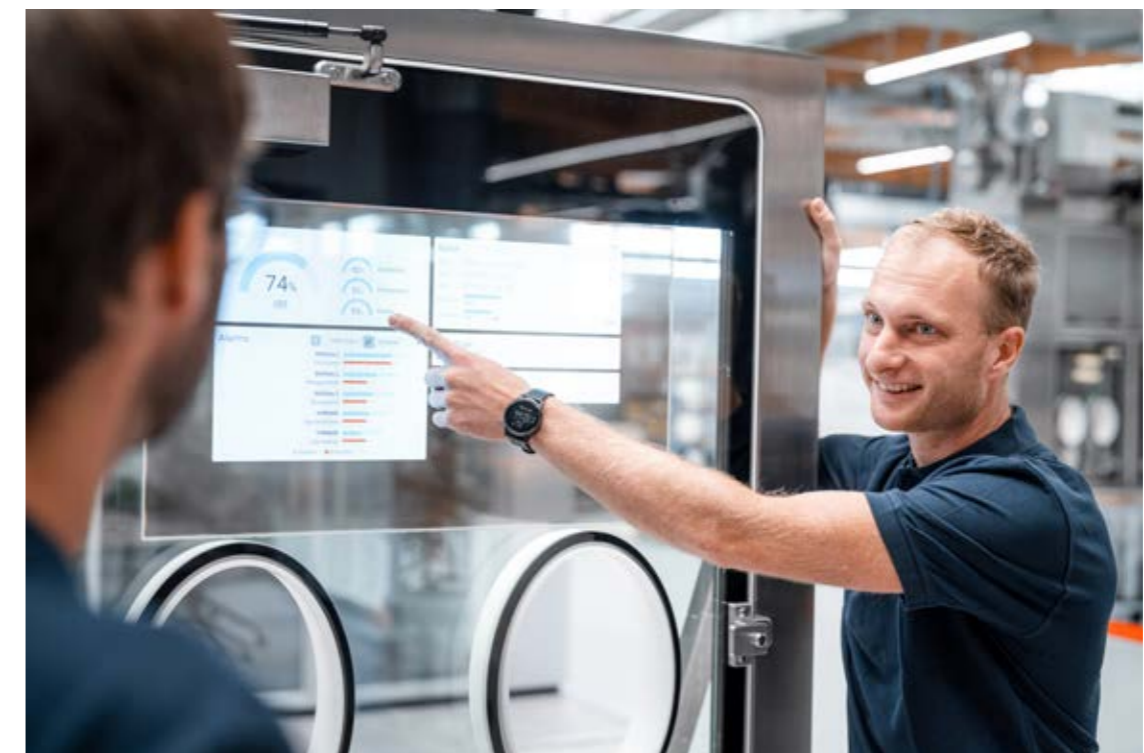
A new type of OLED panel within the isolator pane can be operated and displays information and video instructions. It is transparent when not in use.
