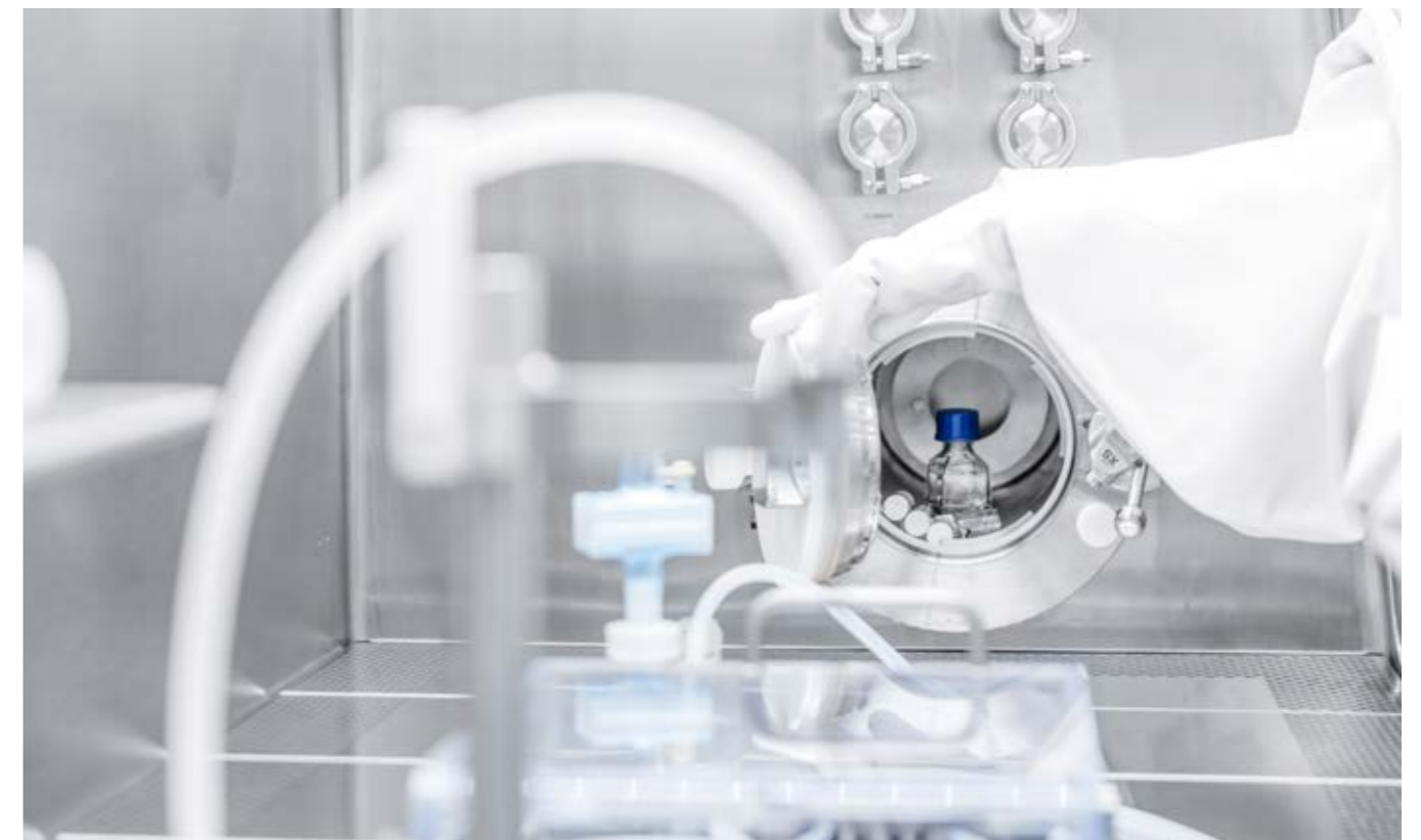
↑ Material transfer via optional RTP port
