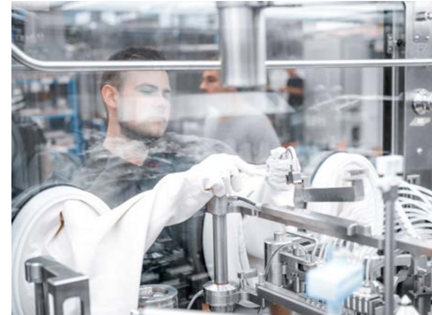
↑ Installing format parts with a simple "click" – Optima designed a special mechanism utilizing customer feedback and extensive testing
