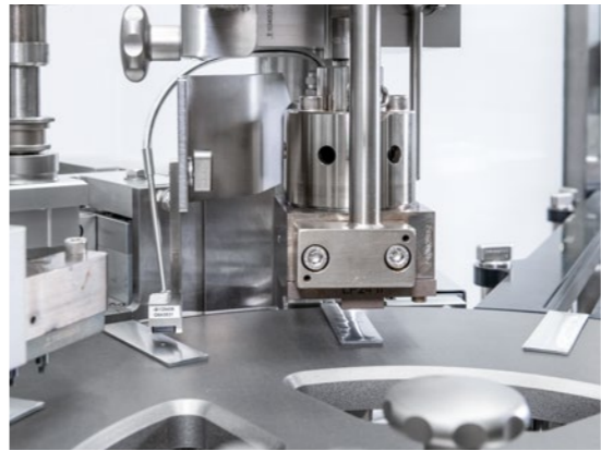
↑ Pre-sealing at four points and then final heat sealing. No waste: 100 Percent of the film is used.
