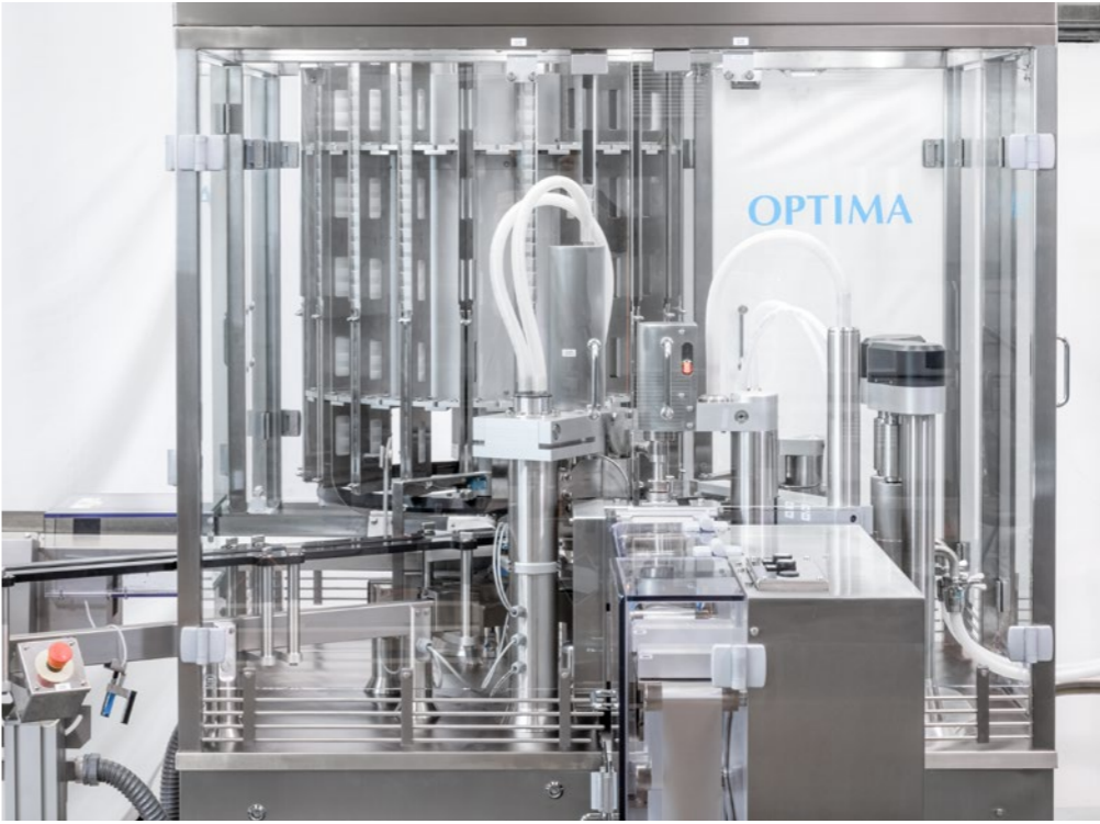
← Part of the updates to the first machine version was a new container magazine. This means the systems can now be operated without interruption.
