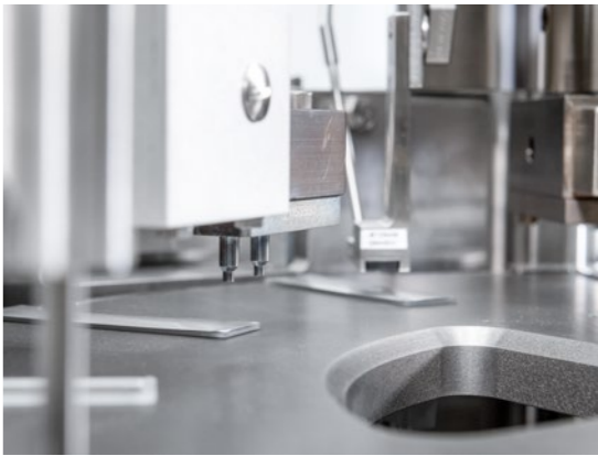
↑ After pre-closing, there is enough time to complete the final heat-sealing with a high output.
