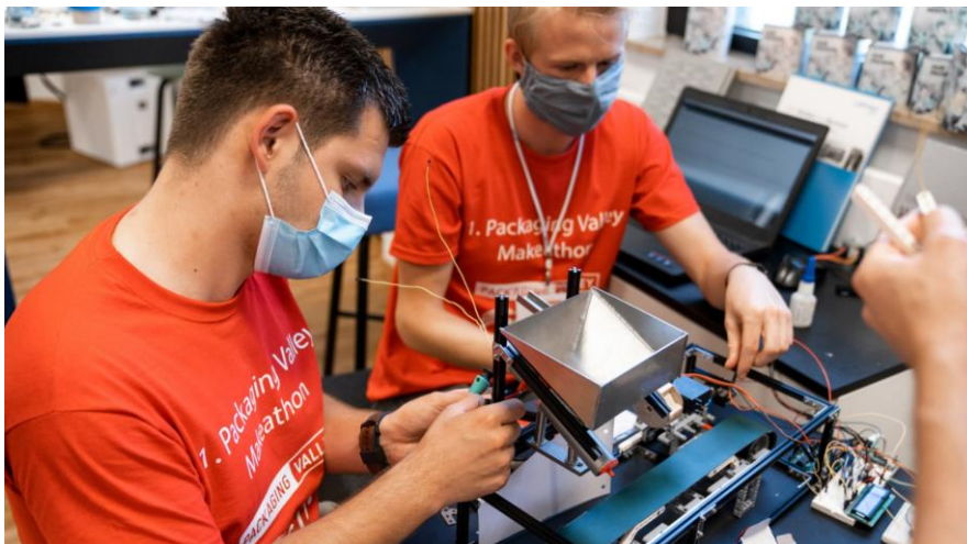
One of the project teams is working on a miniature machine for filling bulk material into returnable containers. (Source: Optima)
