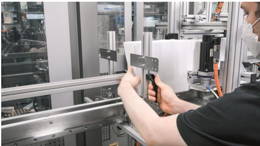
All machine solutions from Optima Nonwovens can be flexibly adapted to different packaging materials. Here, paper bags for packaging sanitary napkins are loaded into the machine. (Source: Optima)
