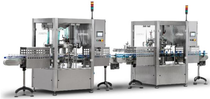
OPTIMA FM1 and CM1 – the flexible entry-level solutions for filling and sealing cosmetic products – can be operated as standalone systems or in line.
