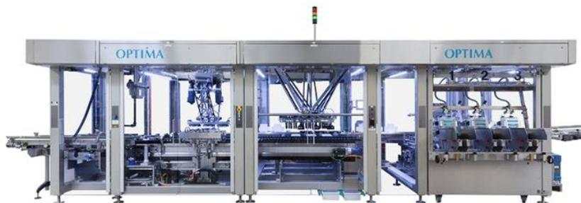
The OPTIMA CBF cartoning machine packs portion packages, for example, into eye-catching, high-quality sales packaging.
