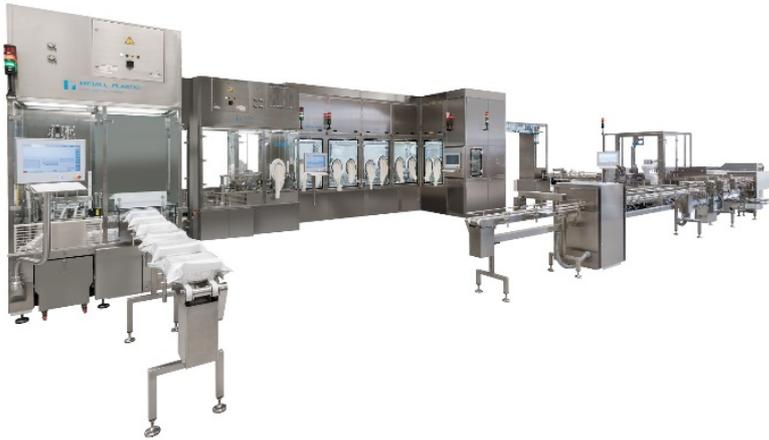
The OPTIMA H6-10 is suited to flexible, high-performance processing. It can handle syringes, cartridges and vials with ease. A variety of different dosage systems can be integrated into the machine.
