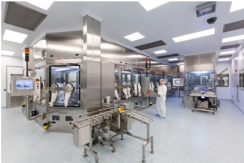
The OPTIMA MultiUse Filler has been specially designed for small to medium batches, as well as for high potency medicines. The modular machine platform also incorporates robot technology for maximum flexibility.
