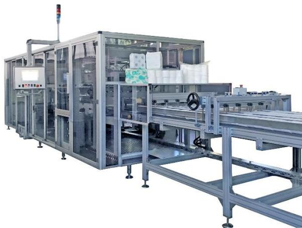
For paper hygiene products: The AMOTEK PB192 delivers highly efficient packaging technology for environmentally friendly packaging of paper, bioplastics and recycled materials. (Source: Amotek/Optima)
